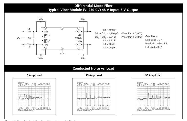
Figure 9–5 — Conducted noise, differential-mode filtering
